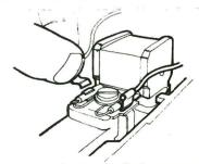
Remove bogie pivot screw. Push power unit forward as far as indicated. Keeping it pushed forward, swivel slightly, at the same time pulling out one side of the under-chassis to release the metal lug (A) from its retaining pegs (B). The power bogie can then easily be removed from the under chassis.
