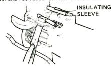
Note: After reassembling power bogie to under-chassis, remember to refit contact wires, anchoring them behind their small retaining pegs, to avoid fouling the body shell. When replacing the latter, remember to fit the front (the end with steps up
